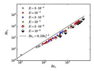
**Fig. 2.** Evolution of the zonal Reynolds number  $Re_z$  as a function of the convective Reynolds number  $Re_c$  in hydrodynamic direct numerical simulations with  $Ra > 10Ra_c, Pr = 1$  and different Ekman numbers. The line gies the 1.3 scaling which appears to fit the low Pr data according to Gillet and Jones (2006). We note that this scaling law also describes our dataset with Pr = 1 in the turbulent regime.
