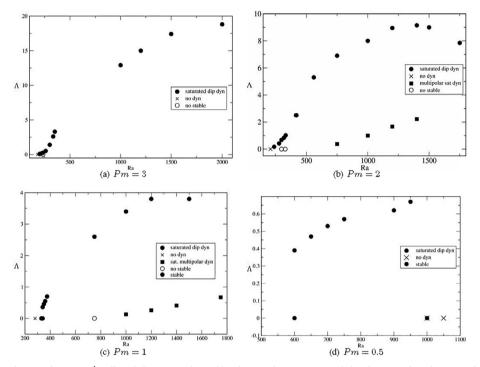
Fig. A.15. Bifurcation dynamo diagrams for  $E = 10^{-4}$ . Full symbols correspond to stable solutions whereas empty symbols refer to initial conditions. Circles are employed for dynamos dominated by the axial dipole component at the surface and squares are employed otherwise.
