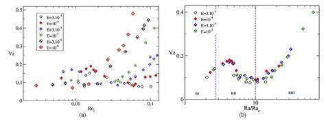
Fig. 1. Relative importance of zonal flows measured by  $V_Z$  in hydrodynamical simulations as a function of  $Ro_\ell$  (panel (a)) and Ra (panel (b)).
