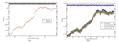
Fig. B.20. Typical behaviour for a multipolar dynamo obtained with a weak initial field. The legend is similar to that of Fig. B.19. The parameters are  $E = 3 \cdot 10^{-4}$ , Pm = 3 and Ra = 650 = 10.69  $Ra_c$ . The magnitude of the initial weak magnetic field is first amplified in the kinematic phase. Then, a non-dipole dominated solution is obtained even if  $Ro_l = 0.091$  and no-slip boundaries are used.
