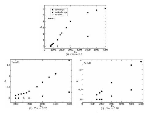
Fig. A.18. Magnetic field strength measured by  $\Lambda$  as a function of the Rayleigh number Ra with  $E=10^{-5}$ . The observed behaviour corresponds to subcritical bifurcations.
