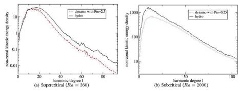
Fig. 10. Kinetic energy distribution of the convective flow (non-zonal) as a function of the harmonic degree l with  $E = 3 \cdot 10^{-5}$ . Dynamo results for dipolar solutions are compared to their associated hydrodynamic models for magnetic Reynolds numbers close to their critical values.
