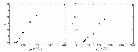
Fig. A.17. Magnetic field strength measured by  $\Lambda$  as a function of the Rayleigh number Ra for dipolar dynamos with  $E=10^{-5}$ . Supercritical bifurcations are observed.
