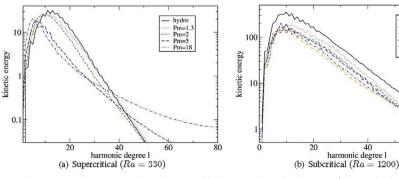
Fig. 11. Kinetic energy distribution of the convective flow (non-zonal) as a function of the harmonic degree l with  $E=10^{-4}$  close to the dynamo threshold for a typical supercritical model (left panel) and a typical subcritical one (right panel). For  $E=10^{-4}$  and P=1, P
