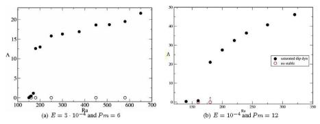
Fig. A.14. Dynamo bifurcation diagrams are shown where empty circles correspond to initial conditions which are not stable. For  $E = 3 \cdot 10^{-4}$  and  $E = 10^{-4}$ , non-magnetic flows are classified as laminar flows with Ra < 220 ( $Ra < 3.62Ra_c$ ) and Ra < 220 ( $Ra < 3.25Ra_c$ ) respectively.
