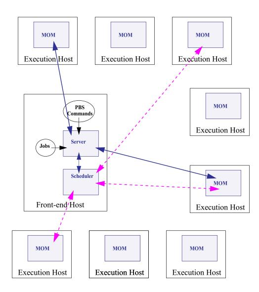
This diagram illustrates a multi-node cluster configuration wherein the Scheduler and Server communicate with the MOMs on the execution nodes. Jobs are submitted to the Server, scheduled for execution by the Scheduler, and then transferred to a MOM when it's time to be run. MOM periodically sends status information back to the Server, and answers resource requests from the Scheduler.
